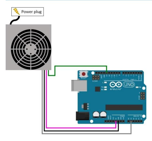
When you call the turnOn() method the power source is turned on, and these wires are powered with a higher amperage:
